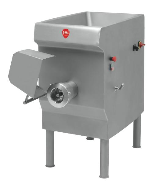
The machine casing can be taken apart very quickly and easily. The smooth surfaces and the swing-away protection of the feeding funnel (equipped with a magnetic security sensor), both make for an easy cleaning of the machine.
